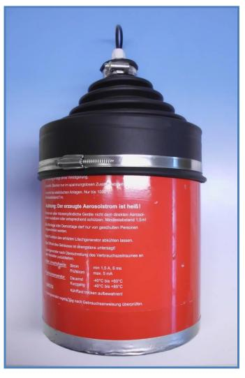
Important: A cable loop of approx. 20 cm must be set into the space between the rubber protection cover and fire extinguishing generator, after connecting the squib connector to the fire extinguishing generator, before the final mounting of the rubber protection cover, so thus the squib connector can't be damaged during operation and during disassembly!
